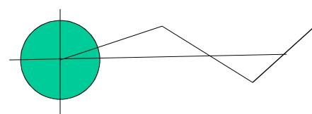
N2 Pressure too <u>high</u>, ->Excessive Roller Movement, Inefficient Grinding, Rough Running
