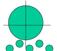
Grinding bed too <u>high</u>, ->Vibration Inefficient Grinding
